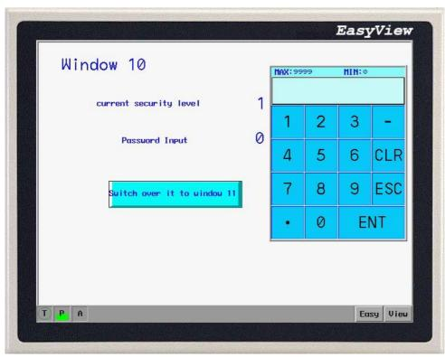
Press the switch window button under security level 1, window is successfully changed to window 11:
