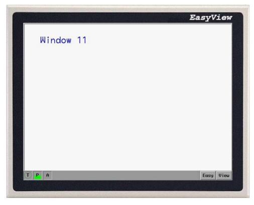
However, how to switch the higher level security to lower lever security? LW9043 allows the project to force the HMI to a lower security level. Add a Numeric Data on window 10 as below:
